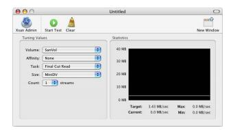
1 When you have selected the volume to test and the test parameters, click Start Test.
