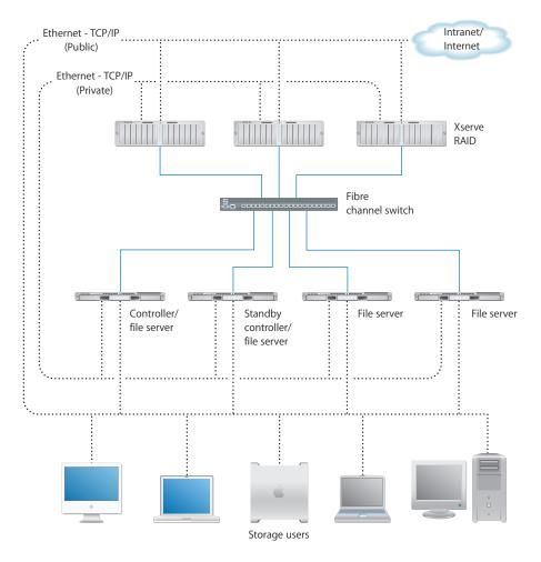
You can use a combination of Xserve and Xserve RAID to provide NAS and, in addition, provide other server services that NAS appliances can't offer. Adding Xsan lets you set up a NAS service that is easy to expand, both in terms of storage capacity and file system services, without impact to clients.
